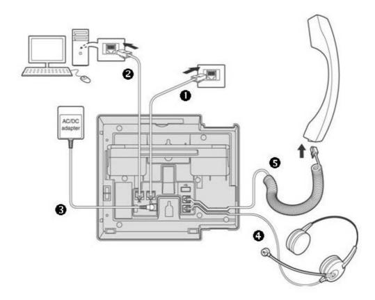
1 LAN Connect the IP Phone LAN port to the LAN wall jack with the provided LAN cable.
